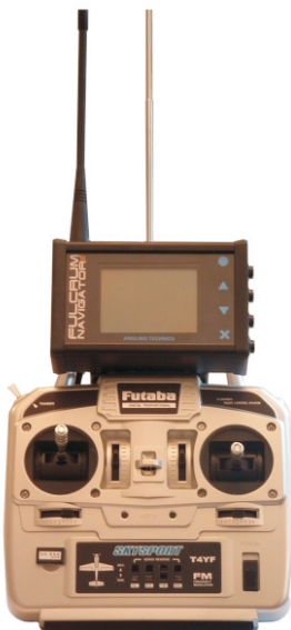
LCD Display Mounted on the Transmitter
